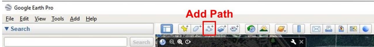
Figure 3. The Google Earth 'Add Path' tool (indicated with a red rectangle) marks the points along a digital path or traverse.
