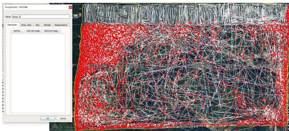
Figure 6. Google Earth image showing the field training course area with the digitised points along traverses. Note that there are gaps between traverses, and other runs are needed to fill in the gaps.
