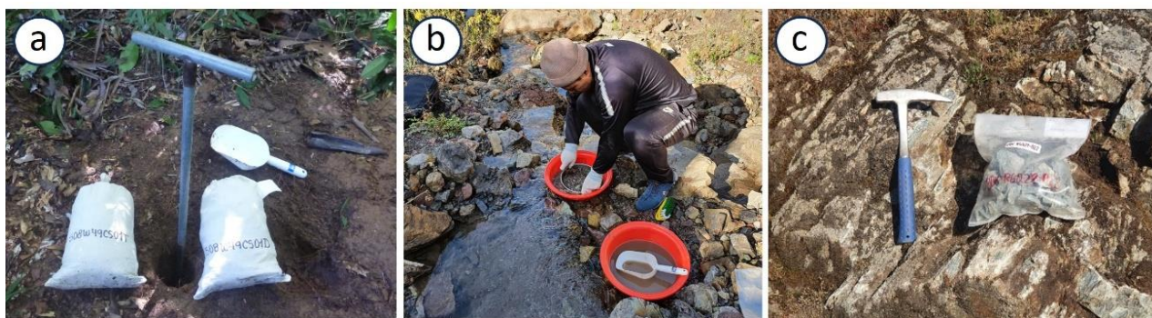
Figure A2.18. Types of sampling carried out in the various studies of the National Geochemistry Programme: (a) Soil sampling; (b) Stream sediment sampling, and (c) Rock sampling.
